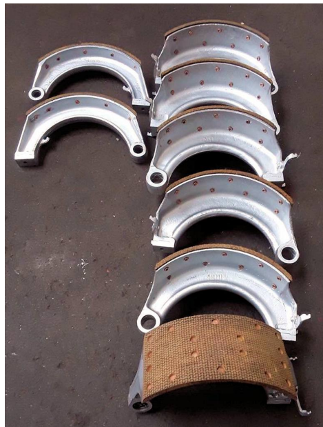
All the refurbished sets of brake shoes are back on site. [Keith Walker]
