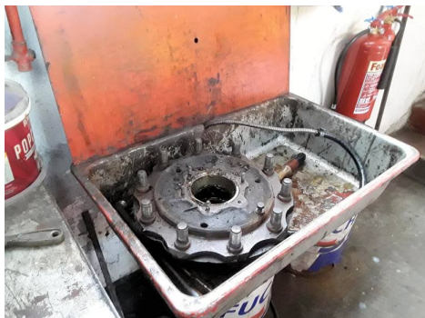
Cardiff 262's front offside hub assembly in the paraffin cleaning tank. [Keith Walker]
